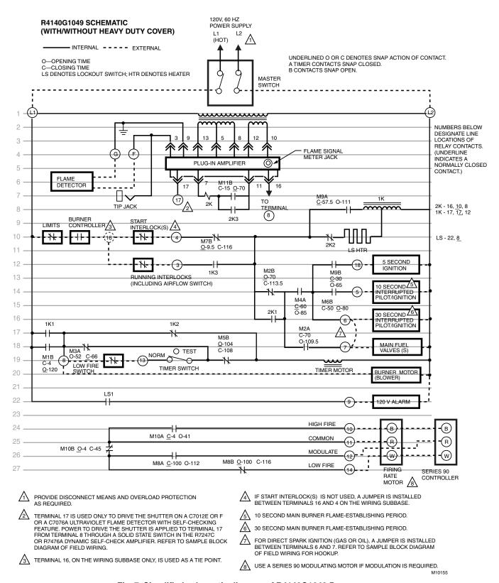
Fig. 7. Simplified schematic diagram of R4140G1049 Programmer.
